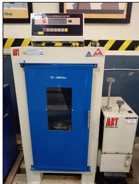
**Gambar 1. 4** *Compression Testing Machine*
