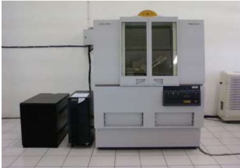
Gambar 30. Difraktometer Sinar-X (Philips X'Pert Powder)
